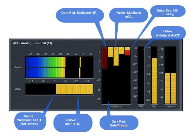
Meters are provided for monitoring input levels, Input AGC, Wideband AGC1, Multiband AGC and Limiters, Multiband Noise Reduction, Multiband Stereo Enhancement, Wideband AGC2 post-multiband output and individual left and right outputs. In the HD section, meters for the final look-ahead peak limiters and the final output of the processing core are added while the AGC output meters are eliminated.
