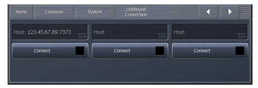
Normally, an instance of NfRemote running on a remote computer initiates the connection to an Omnia.7 ("outbound" connection). However, there are some situations where it is more appropriate for Omnia.7 to initiate the connection to an instance of NfRemote on a remote computer ("inbound" connection).
