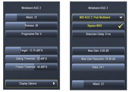
The Wideband AGC 2 menu provides the controls to determine the location and type of compressor as well as all of the expected gain and speed controls.
