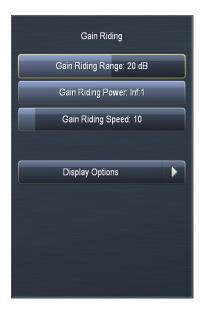
The setting of the Gain Riding Range control affects the Input AGC only and determines the amount of available gain. Setting this control too high may provide too much room for low level audio to be raised up while not providing enough room to adequately attenuate higher input levels. Conversely, setting it too low may not provide enough gain to increase low incoming levels.
