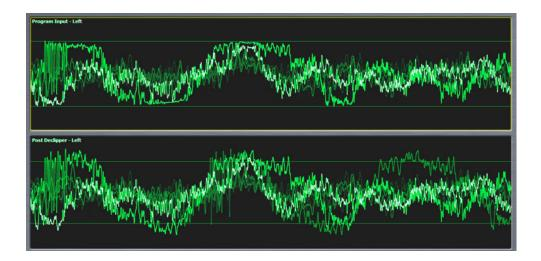
The second stage of Undo is a multi-band expander that is designed to restore dynamic range to audio that has been excessively compressed.
