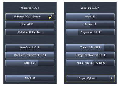
The Wideband AGC1 Enable button enables this compressor, which follows the Input AGC section and provides additional wideband compression as determined by its various controls. Disabling the Wideband AGC1 also makes this patch point unavailable in an oscilloscope or RTA display window.
