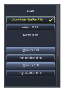
♦ The Volume-based High Pass Filter provides a means by which adjust the high pass filter frequency on the monitor outputs as the volume level is raised. This can help protect smaller monitor speakers by reducing the amount of low frequency energy routed to them at higher listening levels.
