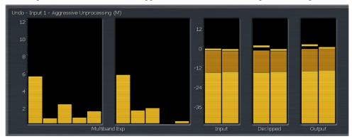
The Dynamics Detectors meters indicate the amount of dynamics detected in each band. Taller bars indicate more inherent dynamics in the source music while shorter bars indicate less dynamics. These meters are generally the inverse of the Expander Ratio meters.
