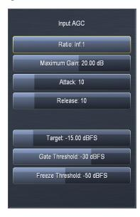
It is worth noting that traditional processors only act upon audio above a particular threshold. They are driven into various amounts of gain reduction, but once the audio falls below the threshold, they "run out of room" or "top out" and are incapable of increasing the audio any further. This necessitates some sort of make-up gain control later in the audio chain.
