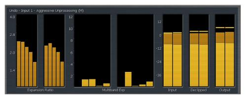
• Undo utilizes a second set of parallel expanders which look at the same input and automatically scale the attack and release characteristics of the main expanders. The **Speed Governor** meters show the activity of these expanders.
