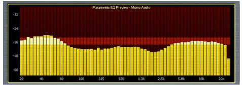
You will now be able to see the curve of the PEQ in the RTA display window. You can also view the curves of each band of the multiband compressor by selecting one of the Solo band buttons. Since the Solo bands relate to a dynamic section of the processing core, lowering the Averages slider will yield more of a "real time" view.
