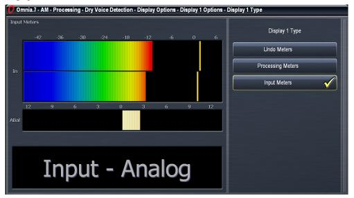
◆ The Input Meters menu allows you to monitor the audio levels entering Omnia.7 with ITU-R BS.1770 bargraph meters.
