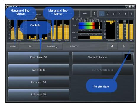
♦ The screen in this view is divided into two sections; the top portion is dedicated to displays while the bottom is reserved for controls. In between these two areas is a navigation bar that shows you exactly where you "are" within Omnia.7 along with navigation arrow buttons that let you go forward or backward to most places you have visited in the fourth tier.
