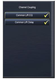
• The Channel Coupling menu provides ganged left and right controls for the EQ and Delay circuits.
