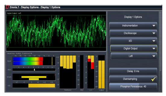
The Category, Patch Point, and Audio Channel sub-menus are used to select the specific source audio. The specific patch points will change depending upon the category. Categories include I/O, Undo, Physical Inputs, Sidechains, Multiband, and Monitor Out.
