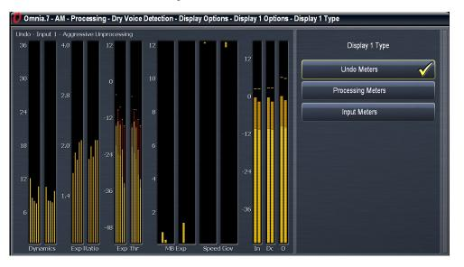
• The Processing Meters menu allows you to display the levels and activity of Omnia.7's various gain stages and processing sections. A complete explanation of these meters is provided in Chapter 6.
