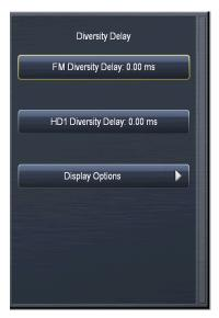
It is also possible to delay the HD-1 audio with the HD Diversity Delay slider. Delaying the HD1 signal by 2 seconds will provide the most accurate and seamless operation of Omnia.7's Speech Detection circuit.
