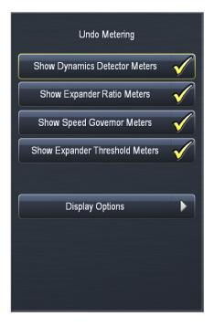
When enabled, the Show Dynamics Detector Meters, Show Expander Ratio Meters, Show Speed Governor Meters, and Show Expander Threshold Meters allow the associated meters for each respective section to be displayed in the Undo Meters window.
