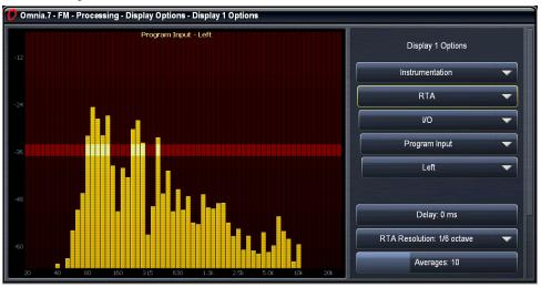
The Category, Patch Point, and Audio Channel sub-menus are used to select the specific source audio. The specific patch points will change depending upon the category. Categories include I/O, Undo, Physical Inputs, Parametric EQ Preview, Sidechains, Multiband, and Monitor Out.
