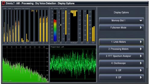
Since the amount of screen "real estate" available for each display decreases as additional windows are added, six available Memory Slots can be set up in different display configurations allowing you to choose which processing parameters or visualizations from one of Omnia.7's valuable built-in diagnostic tools are viewable in each window.
