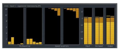
The Expander Threshold meters simultaneously show four different measurements about expander activity. The bright yellow bars indicate the average levels; the orange bars indicate the peak levels; the dark red bars indicate the distance limit (the greatest distance by which an individual band's peak detector can fall relative to the wideband level to prevent any one band from being expanded if there are insufficient levels to begin with); the yellow "blips" indicate peaks.
