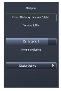
A setting of Level 5 the "normal" setting and recommended for most modern material which have been mastered with high levels of compression and clipping. If your station primarily plays source material that has been cleanly mastered, you may find lower settings are sufficient.
