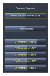
The Downward Expanders operate in a manner similar to a traditional "noise gate" and provide a useful means for reducing unwanted background noise from less-than-perfect program material or from a noisy studio environment. The ratio of the expanders is 2:1.
