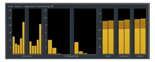
The Expander Ratio meters indicate the current ratio of expansion relative to the detected incoming dynamics. Less dynamic source material will have a higher expander ratio compared to content that is more dynamic.
